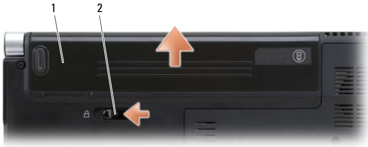
1 battery 2 battery release latch
